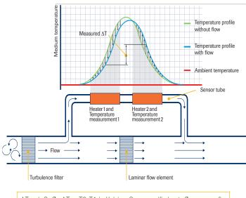
$\Delta T = k.C. \emptyset \Delta T = T2-T1$  in Kelvin  $C_{n} = \text{specific heat } \emptyset_{n} = \text{mass flow}$
